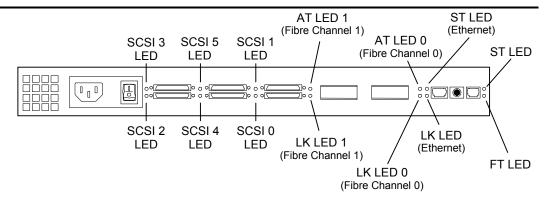
Figure 5-1 Rear View of the Type B Fibre Channel Bridge/Router (FCO)
